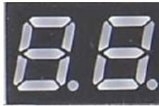
Debug LED with CPU Temperature Monitor
