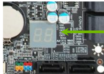
Debug LED with CPU Temperature Monitor
