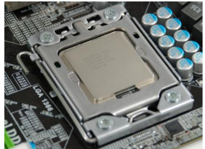
Align notches with notches on the CPU
