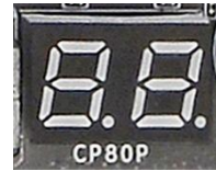
Debug LED with CPU Temperature Monitor
