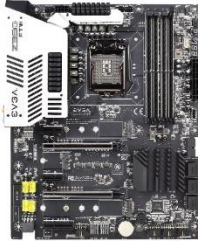
The EVGA Z390 FTW Motherboard This motherboard contains the Intel® B360 chipset.
