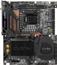
The EVGA Z590 DARK Motherboard This motherboard contains the Intel® Z590 chipset.
