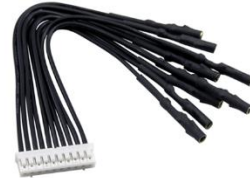
Probel Connector Attach your DMM to the Probel header on the Z690 DARK for real-time voltage measurements.
